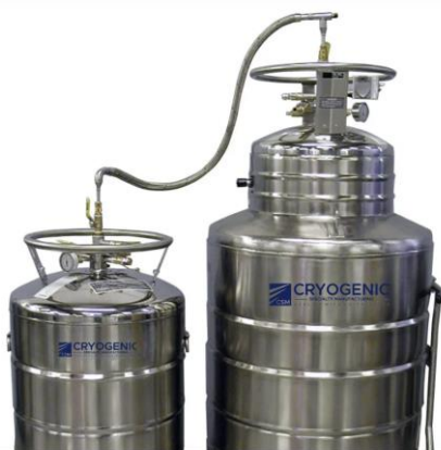
He-Flex is frequently used for Liquid Helium transfer
